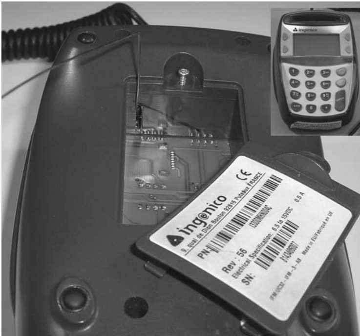
Figure 10.4: A rigid wire is inserted through a hole in the Ingenico’s concealed compartment wall to intercept the smartcard data. The front of the device is shown on the top right.
