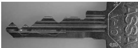
Figure 11.2: Key for a sidebar lock
